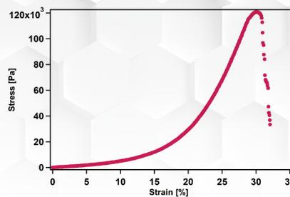
**Figure 4:** Typical compression stress-strain curve of a disc-shaped Collink.3D™ 90 construct, prepared from 1.6 mL Collink.3D™ 90 exposed to 365 nm irradiation for 2 min.
