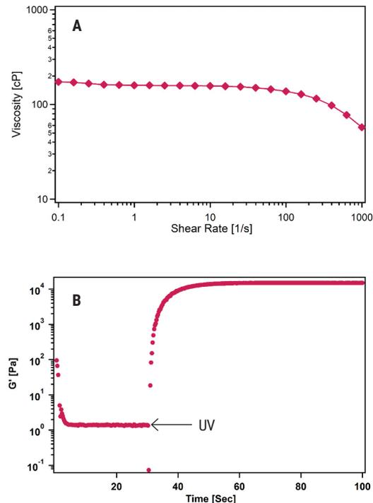
**Figure 3:** Rheological characterization of a 10 mg/mL Collink.3D™ 90 solution in 10 mM HCl. A: Viscosity measurement using the rotation flow sweep test method. B: Curing kinetics measurement at 365 nm irradiation (50 mW/cm<sup>2</sup>), using the oscillation time sweep test method and 0.1% LAP as a photoinitiator.
